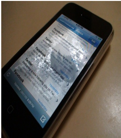
Figure 12: Water damage behind cover glass of iPod.
