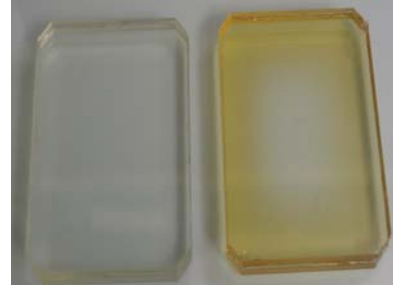
Figure 9: Examples of two different bonding technologies after thermal cycling. Left: No yellowing (96.5% transmittance). Right: Yellowing (85.3% transmittance).
