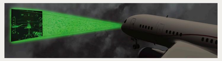
Penetrating deep into weather-shrouded environments, the HVS's multispectral, infrared EVS provides real-time images of the airport environment and obstacles, including vehicles, animals, aircraft and LED runway lighting. Aircraft sensors and navigation data integrate from on-board avionics to execute guidance cues and overlay SVS terrain data as the approach is flown.
