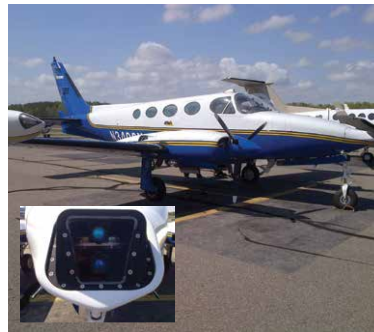
Engineers had to think outside the box to come up with a method for demonstrating our latest night vision technology. Their solution involved placing the ISIE 11 sensor on the front of a twin-propeller Cessna aircraft and modifying the pilot's F-35 HMDS to receive output from the sensor.
