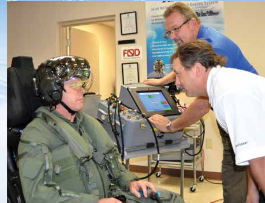
As part of the helmet-fitting process, Dan Kalsow (back) and Rodney Breuer (front) test to ensure the pilot's pupils are within 2 millimeters of exact center to be properly aligned with the optics package on the HMDS.
