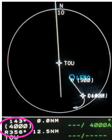
Figure 3a. “Climb to 4000 feet followed immediate by Right turn 356° course to TOU.
