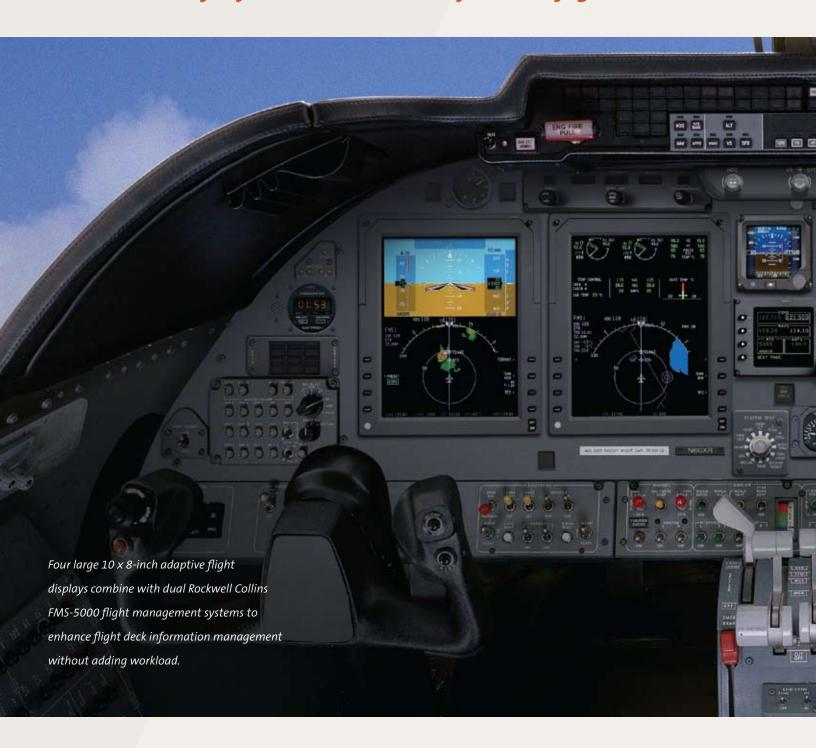
Combining the latest-technology sensors and displays in an integrated package that is both smaller and lighter than traditional avionics, the Rockwell Collins Pro Line 21 suite for the Bombardier Learjet 60 XR is a breakthrough in flight deck efficiency and pilot workload reduction.
