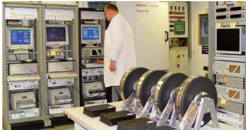
Design and development of our space wheels includes creating the housing assembly (top) and conducting tests on our wheels and their electronic components (bottom).
