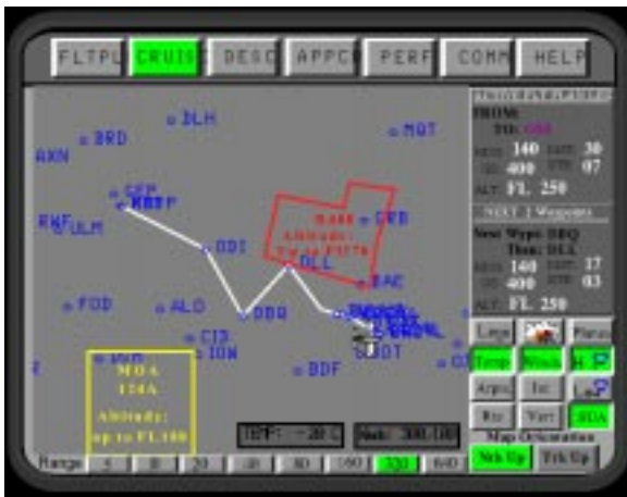
Figure 4. Example of selecting icons to rapidly manipulate the GUI FMS display format
